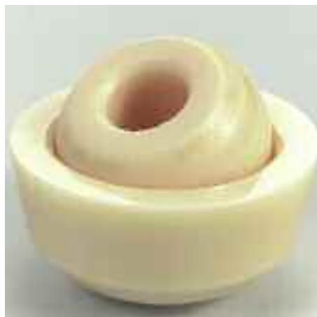
The surfaces of the cup and ball head in a hip joint rub against one another continuously during walking
